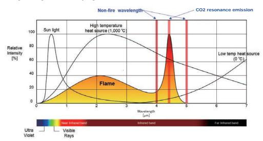
Fire (flame) has a characteristic peak at 4.4  $\mu$ m in a spectral distribution, which is called as CO2 emission. The DRD2-W has 3 sensors that monitor the band of CO2 emission and two wavebands on either side respectively. The detector avoids false alarms by the feature of frequency-fluctuation detection.
