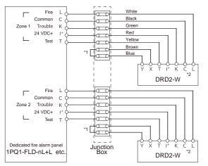
\*1 Install a wire jumper between the terminals connected to Brown and Blue wires. \*2 The DRD2-W has a built-in End-of-Line device (CRE) in its enclosure.
