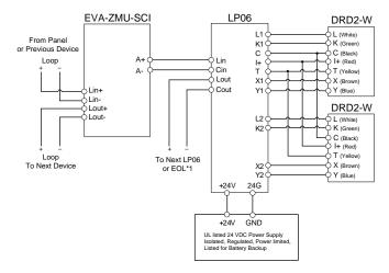
\*1 A 10 kΩ End-of-Line Resister must be installed at the last LP06 in the A+ and A- circuit.
