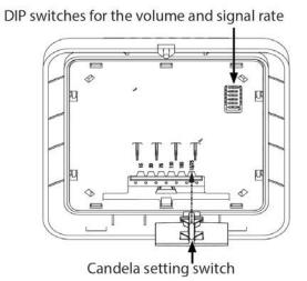
Device settings are located on the back of the unit to prevent tampering
