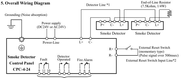
Non-Voltage C Contact: The labels indicate a condition when power is supplied.
